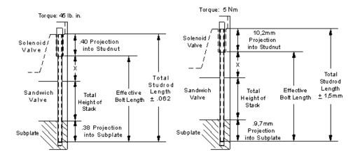
To simplify the installation of ISO 03 and ISO 05 sandwiches, Sun offers uncut (can be cut to length in the field) or precut studkits in both inch and metric standard threaded rod. Once the rods are installed in a subplate or manifold, they act as a guide in assembling the sandwich body stack. After the directional control valve is assembled on top of the stack, Sun studnuts are used to retain the assembled stack.
