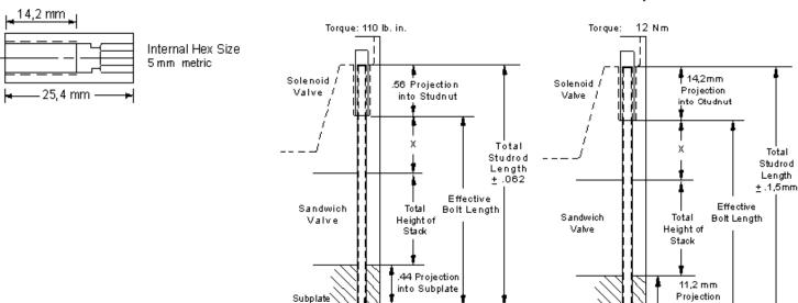
To simplify the installation of ISO 03 and ISO 05 sandwiches, Sun offers uncut (can be cut to length in the field) or precut studkits in both inch and metric standard threaded rod. Once the rods are installed in a subplate or manifold, they act as a guide in assembling the sandwich body stack. After the directional control valve is assembled on top of the stack, Sun studnuts are used to retain the assembled stack.
