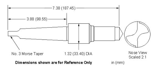
Morse taper form drills and reamers are available for machining Sun cavities.
