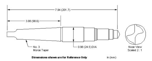
Morse taper form drills and reamers are available for machining Sun cavities.
