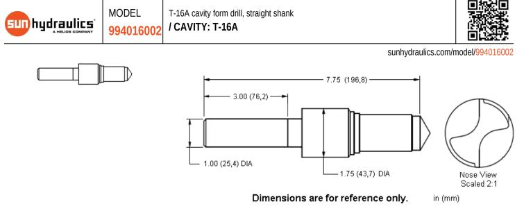
Straight shank form drills and reamers are available for machining Sun cavities.
