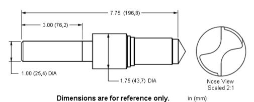
Straight shank form drills and reamers are available for machining Sun cavities.
