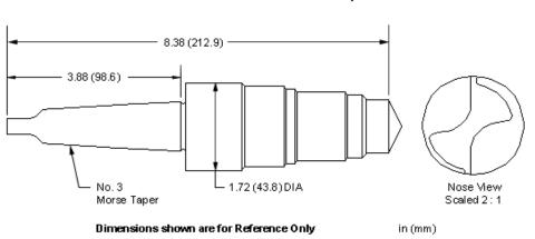
Morse taper form drills and reamers are available for machining Sun cavities.
