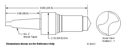
Morse taper form drills and reamers are available for machining Sun cavities.
