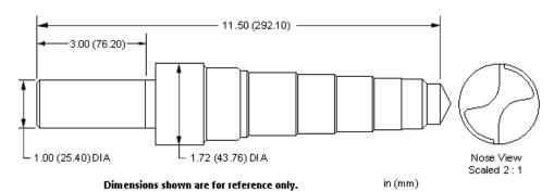
Straight shank form drills and reamers are available for machining Sun cavities.
