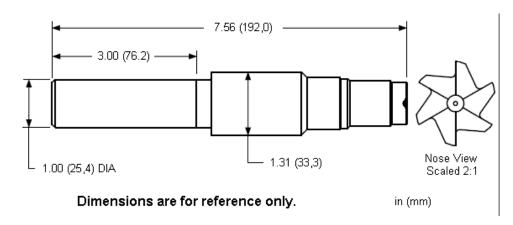
Straight shank form drills and reamers are available for machining Sun cavities.
