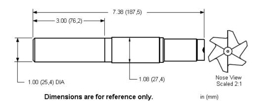
Straight shank form drills and reamers are available for machining Sun cavities.
