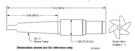
Morse taper form drills and reamers are available for machining Sun cavities.
