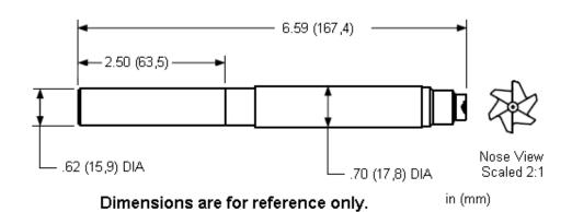
Straight shank form drills and reamers are available for machining Sun cavities.
