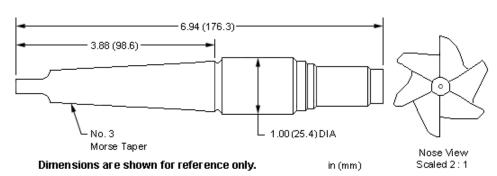
Morse taper form drills and reamers are available for machining Sun cavities.
