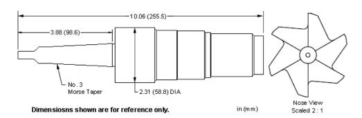
Morse taper form drills and reamers are available for machining Sun cavities.
