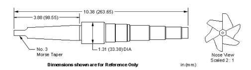
Morse taper form drills and reamers are available for machining Sun cavities.
