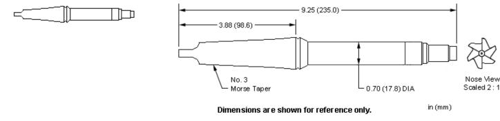
Morse taper form drills and reamers are available for machining Sun cavities.
