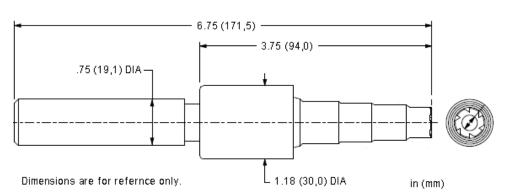
$\textbf{NOTES:} \quad \bullet \quad \text{All diameters are concentric within .0005 T.I.R.}$
