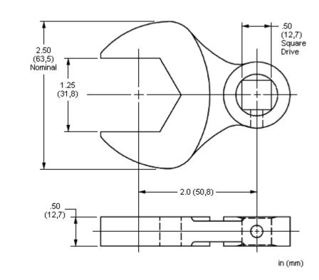
This tool is used to install Series 3 LO\*\* and LK\*\* cartridges equipped with the Z control (position indicating switch).
