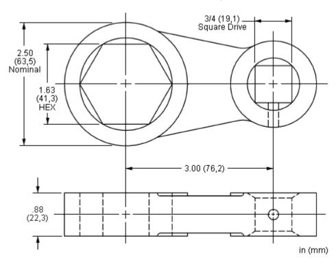
This tool is used to install Series 4 LO\*\* and LK\*\* cartridges equipped with the Z control (position indicating switch).
