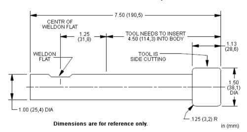
This tool is used to generate the annulus, or undercut, for optimized T-18AU and T-19AU Series 4 Plus cavities.
