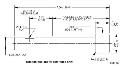
This tool is used to generate the annulus, or undercut, for optimized T-18AU and T-19AU Series 4 Plus cavities.
