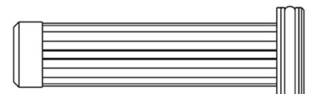
Replaceable filter elements are available for Sun's line of filter cartridges. These include surface type (last chance) and depth style elements. See the Technical Data tab for details on this element.
