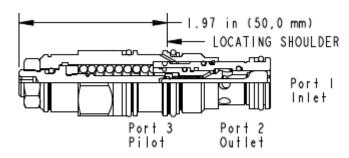
Counterbalance valves with pilot assist are meant to control an overrunning load. The check valve allows free flow from the directional valve (port 2) to the load (port 1) while a direct-acting, pilot-assisted relief valve controls flow from port 1 to port 2. Pilot assist at port 3 lowers the effective setting of the relief valve at a rate determined by the pilot ratio. Other names for this valve include motion control valve and over-center valve.
