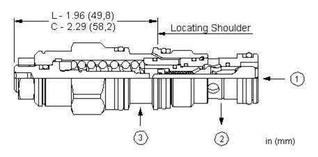
Counterbalance valves with pilot assist are meant to control an overrunning load. The check valve allows free flow from the directional valve (port 2) to the load (port 1) while a direct-acting, pilot-assisted relief valve controls flow from port 1 to port 2. Pilot assist at port 3 lowers the effective setting of the relief valve at a rate determined by the pilot ratio. Other names for this valve include motion control valve and over-center valve.
