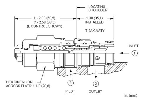
Counterbalance valves with pilot assist are meant to control an overrunning load. The check valve allows free flow from the directional valve (port 2) to the load (port 1) while a direct-acting, pilot-assisted relief valve controls flow from port 1 to port 2. Pilot assist at port 3 lowers the effective setting of the relief valve at a rate determined by the pilot ratio. Other names for this valve include motion control valve and over-center valve.
