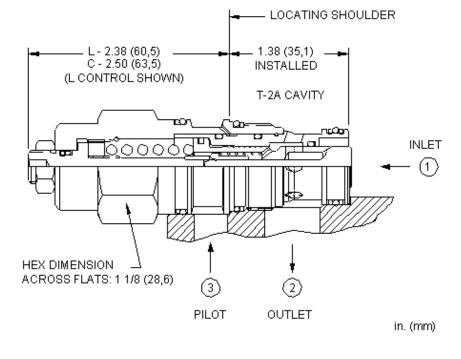
Counterbalance valves with pilot assist are meant to control an overrunning load. The check valve allows free flow from the directional valve (port 2) to the load (port 1) while a direct-acting, pilot-assisted relief valve controls flow from port 1 to port 2. Pilot assist at port 3 lowers the effective setting of the relief valve at a rate determined by the pilot ratio. Other names for this valve include motion control valve and over-center valve.
