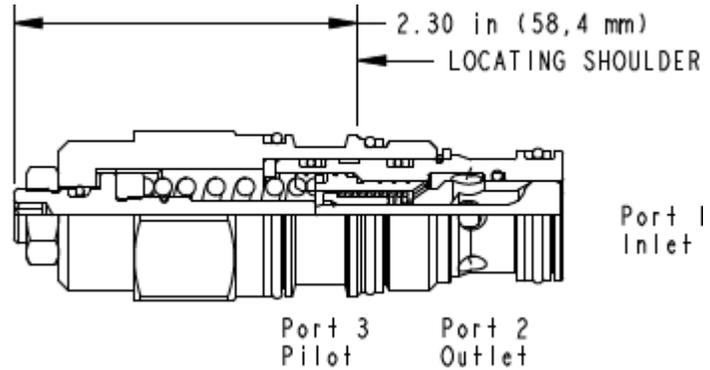
Counterbalance valves with pilot assist are meant to control an overrunning load. The check valve allows free flow from the directional valve (port 2) to the load (port 1) while a direct-acting, pilot-assisted relief valve controls flow from port 1 to port 2. Pilot assist at port 3 lowers the effective setting of the relief valve at a rate determined by the pilot ratio. Other names for this valve include motion control valve and over-center valve.
