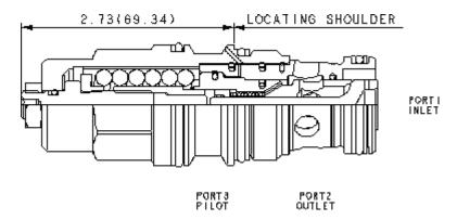
Counterbalance valves with pilot assist are meant to control an overrunning load. The check valve allows free flow from the directional valve (port 2) to the load (port 1) while a direct-acting, pilot-assisted relief valve controls flow from port 1 to port 2. Pilot assist at port 3 lowers the effective setting of the relief valve at a rate determined by the pilot ratio. Other names for this valve include motion control valve and over-center valve.
