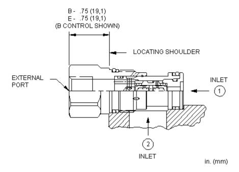
The back-to-back check valve combines two simple check valves into a single cartridge. It connects the higher of two work ports to the signal or common port. The signal is sensed at an external port located in the hex-end of the cartridge.
