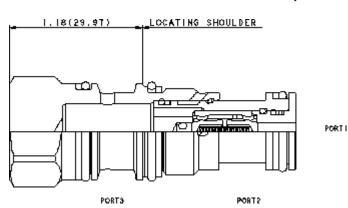
The back-to-back check valve combines two simple check valves into a single cartridge. It connects the work port with the higher pressure to the signal or common port. The signal is sensed at port 3.
