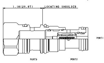
The back-to-back check valve combines two simple check valves into a single cartridge. It connects the work port with the higher pressure to the signal or common port. The signal is sensed at port 2.
