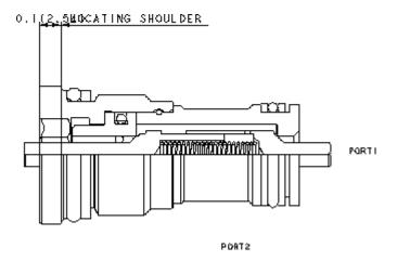
The phaser check is a pair of checks, back-to-back, with both poppets mechanically actuated. The valve is meant to be installed into the piston or rod of a cylinder. When the cylinder reaches the end of its stroke the poppet in the phaser check is shoved off its seat allowing flow through the piston. This allows two cylinders to get back into phase.
