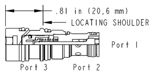
This valve is a pilot to open check valve. It has a sealed pilot, a steel seat, and is non-vented. It allows free flow from the valve (port 2) to the load (port 1) and blocks flow in the opposite direction. Pressure at the pilot (port 3) will open the valve from port 1 to port 2. Pilot pressure needed at port 3 to open the valve is directly proportional to the load pressure at port 1. Pressure at port 2 directly opposes pilot pressure.
