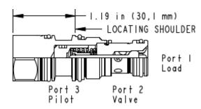
This valve is a pilot to open check valve. It has a non-sealed pilot, a steel seat, and is non-vented. It allows free flow from the valve (port 2) to the load (port 1) and blocks flow in the
