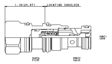
This valve is a pilot to open check valve. It has a non-sealed pilot, a steel seat, and is non-vented. It allows free flow from the valve (port 2) to the load (port 1) and blocks flow in the opposite direction. Pressure at the pilot (port 3) will open the valve from port 1 to port 2. Pilot pressure needed at port 3 to open the valve is directly proportional to the load pressure at port 1. Pressure at port 2 directly opposes pilot pressure.
