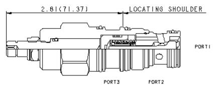
This valve is a pilot to open check valve. It has a non-sealed pilot, a steel seat, and is non-vented. It allows free flow from
