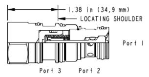
This valve is a pilot to open check valve. It has a non-sealed pilot, a steel seat, and is non-vented. It allows free flow from the valve (port 2) to the load (port 1) and blocks flow in the opposite direction. Pressure at the pilot (port 3) will open the valve from port 1 to port 2. Pilot pressure needed at port 3 to open the valve is directly proportional to the load pressure at port 1. Pressure at port 2 directly opposes pilot pressure.
