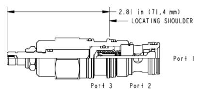
This valve is a pilot to open check valve. It has a sealed pilot, a Delrin seat, and is non-vented. It allows free flow from the valve (port 2) to the load (port 1) and blocks flow in the opposite direction. Pressure at the pilot (port 3) will open the valve from port 1 to port 2. Pilot pressure needed at port 3 to open the valve is directly proportional to the load pressure at port 1. Pressure at port 2 directly opposes pilot pressure.
