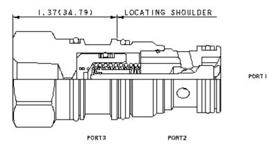
This valve is a pilot to open check valve. It has a sealed pilot, a steel seat, and is non-vented. It allows free flow from the
