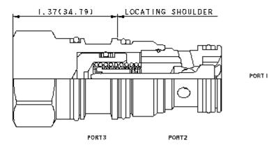
This valve is a pilot to open check valve. It has a sealed pilot, a steel seat, and is non-vented. It allows free flow from the valve (port 2) to the load (port 1) and blocks flow in the opposite direction. Pressure at the pilot (port 3) will open the valve from port 1 to port 2. Pilot pressure needed at port 3 to open the valve is directly proportional to the load pressure at port 1. Pressure at port 2 directly opposes pilot pressure.
