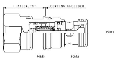
This valve is a pilot to open check valve. It has a non-sealed pilot, a steel seat, and is vented. It allows free flow from the
