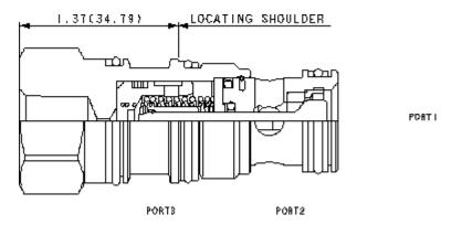
This valve is a pilot to open check valve. It has a non-sealed pilot, a steel seat, and is vented. It allows free flow from the
