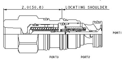
This valve is a pilot to open check valve. It has a sealed pilot, a steel seat, and is vented. It allows free flow from the valve (port 2) to the load (port 1) and blocks flow in the opposite
