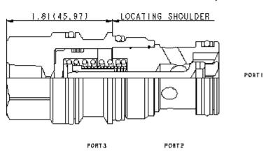
This valve is a pilot to open check valve. It has a non-sealed ree flow from the valve (port 2) to the load (port 1) and blocks flow
