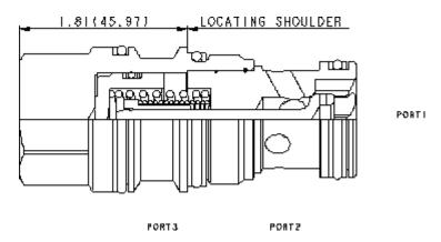
This valve is a pilot to open check valve. It has a sealed pilot, a steel seat, and is non-vented. It allows free flow from the valve (port 2) to the load (port 1) and blocks flow in the opposite direction. Pressure at the pilot (port 3) will open the valve from port 1 to port 2. Pilot pressure needed at port 3 to open the valve is directly proportional to the load pressure at port 1. Pressure at port 2 directly opposes pilot pressure.
