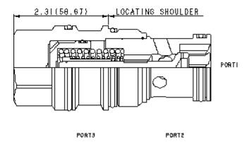
This valve is a pilot to open check valve. It has a sealed pilot, a steel seat, and is non-vented. It allows free flow from the valve (port 2) to the load (port 1) and blocks flow in the opposite direction. Pressure at the pilot (port 3) will open the valve from port 1 to port 2. Pilot pressure needed at port 3 to open the valve is directly proportional to the load pressure at port 1. Pressure at port 2 directly opposes pilot pressure.
