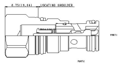
This valve is a fixed-orifice, non-pressure-compensated flow control with a reverse flow check. The flow setting is specified by the user and is set at the factory.
