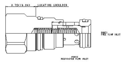
Free-flow, nose-to-side check valves with a bypass orifice allow free flow from port 1 to port 2. A customer specified orifice is included to restrict flow from port 2 to port 1. See technical data below for orifice range.
