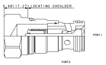
This valve is a fixed-orifice, non-pressure-compensated flow control with a reverse flow check. The flow setting is specified by the user and is set at the factory.
